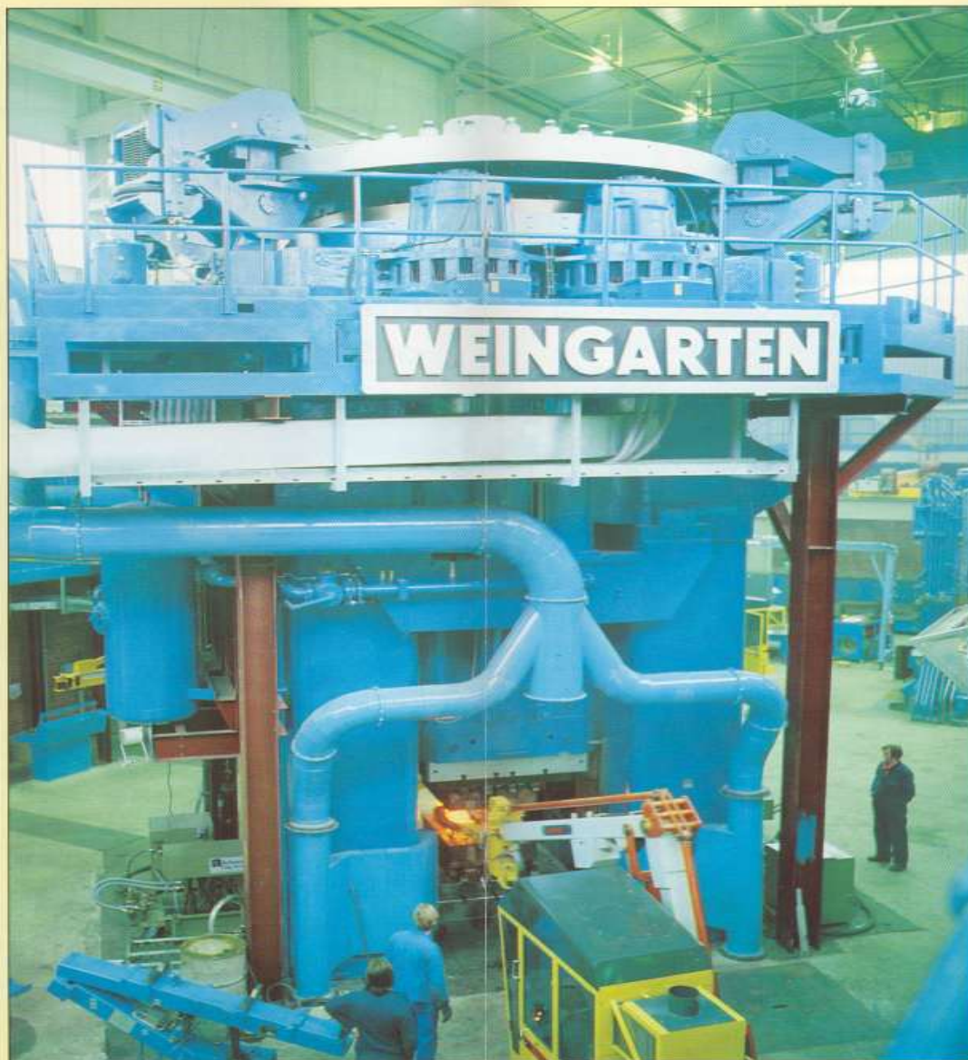
The 16,000 Tonne Weingarten Percussion Screw Press.
